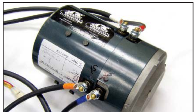
11d, f, g & h. Cable Installation on Motor
